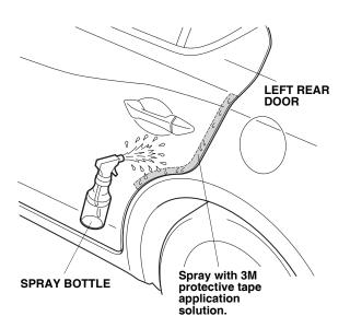
Open the left rear door. Peel back about 50 mm (2.0 in.) of adhesive backing from the left rear door edge film. Align the V-notch 30 mm (1.2 in.) above the character line on the upper part of the left rear door as shown.
