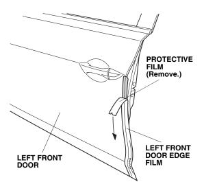
7. Starting from the center and working outward, use your fingers to fold the left front door edge film around the edge of the left front door. Move your fingers in one direction. Attach the door edge film over the seam sealant. Do not trim or damage the seam sealant.
