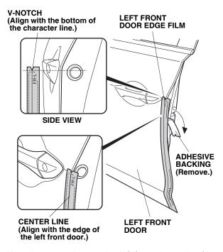
Align the center line on the left front door edge film with the edge of the left front door. While applying light pressure, carefully remove the adhesive backing, and attach the left front door edge film to the left front door. 5. Insert the applicator into the soft sleeve. Starting from the top and working downward, use the soft sleeve to smooth the left front door edge film. Move the soft sleeve in one direction only.
