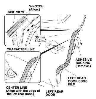
11. Align the center line on the left rear door edge film with the edge of the left rear door. While applying light pressure, carefully remove the adhesive backing, and attach the left rear door edge film to the left rear door.
