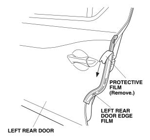
14. Starting from the center and working outward, use your fingers to fold the left rear door edge film around the edge of the left rear door. Move your fingers in one direction. Attach the film over the seam sealant. Do not trim or damage the seam sealant.
